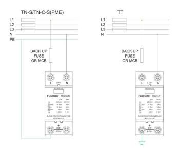
Before powering up the installation check all connections are TORQUED to 2.5Nm. Loose connections cause fires!
