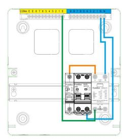
TAIL CLAMP (ACCF) CANNOT BE USED WHEN SPDCUKITT1 IS INSTALLED within a FuseBox consumer unit, unless an additional mounting hole is drilled by the installer for the clamp to be fixed.
